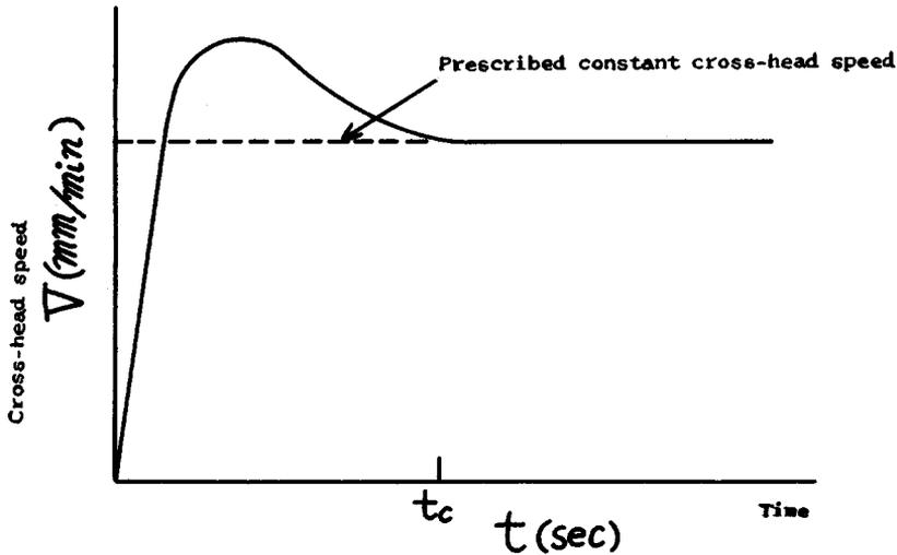
Fig. 2. Cross-head speed vs. time curve (critical damping type).
