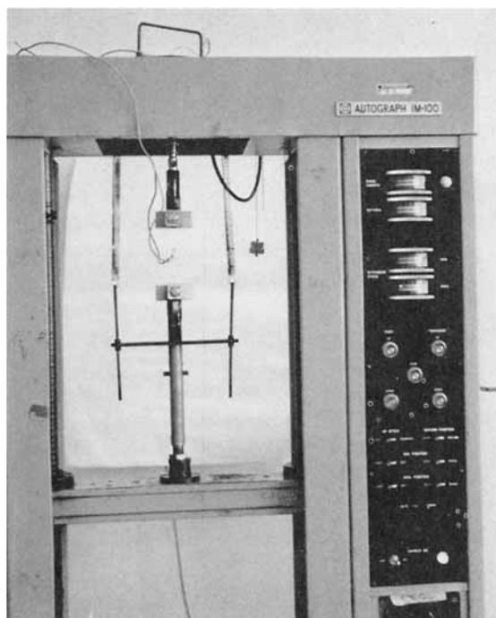
Fig. 5. Setup of IM-100 tensile tester with "slack grip."
