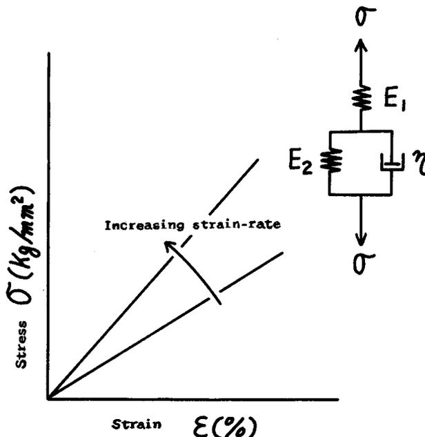
Fig. 4. Stress-strain curve of three-parameter model, showing strain rate dependence.
