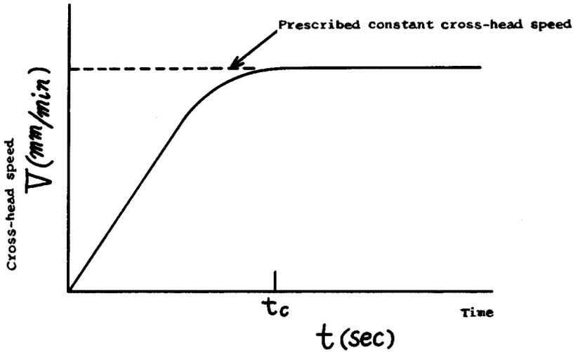
Fig. 1. Cross-head speed vs. time curve (over damping type).
