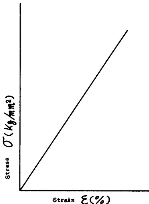
Fig. 3. Stress-strain curve of perfectly elastic material for any strain rate.
