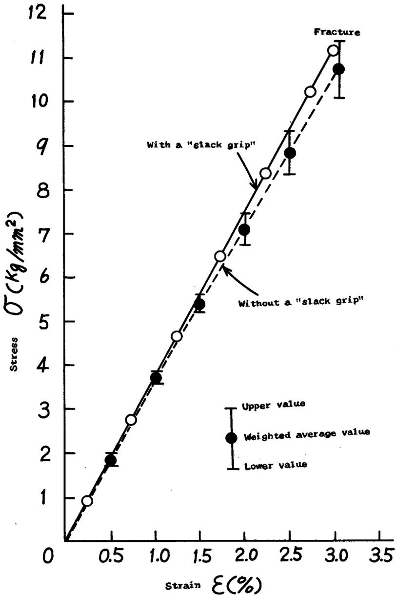
Fig. 6. Experimental results with and without "slack grip."
